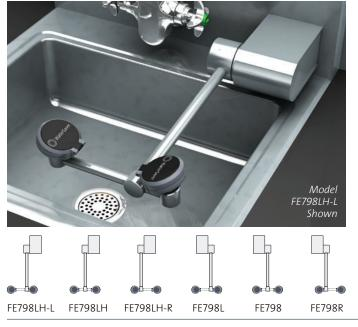
**Application:** Stainless steel AutoFlow™ eye/face wash for mounting on wall behind sink. Water flow is activated by swinging the spray head assembly down over sink.
